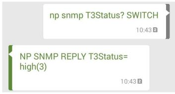
An example of sending an SMS command to switch a logic level of an IO line № 3 in the mode «**output**» with a successful result of completion
