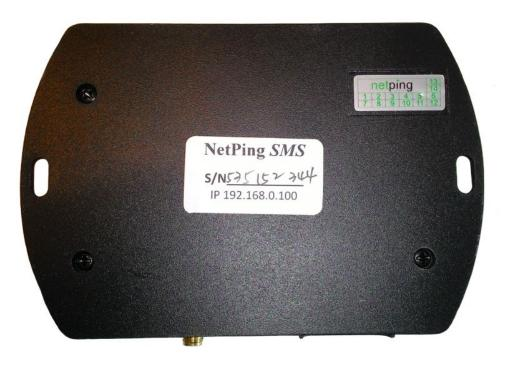
A default IP address of a device is 192.168.0.100
