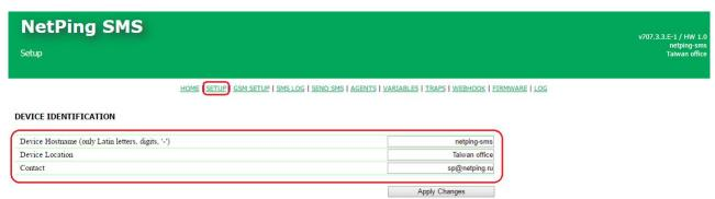
In the section «**Device Identification**», it is possible to configure:
