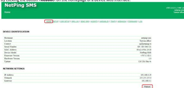
When clicking the button «**Reboot**» a CPU LED near an Ethernet port will blink. A device will reboot.
