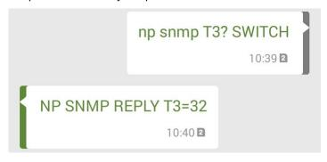
An example of sending an SMS command for receiving the status of a temperature sensor №3 with a successful result of completion:
