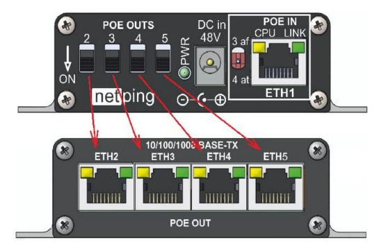
The maximum power consumed by the switch GB332 (and by all the PoE consumers connected to it) must not exceed 30W in accordance with the 802.3at standard. Consumers can be located behind different ports GB322 or behind a single port, there is no restrictions on the total power per port. The maximum power consumption of the switch inself is 7W, it can give the possibility to chain up to 4 switches GB332, using short patch-cords.
